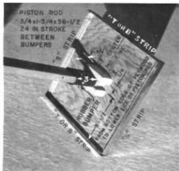
Fig. 14. Plywood Piston with Sheetmetal Sealing Strips Attached.
