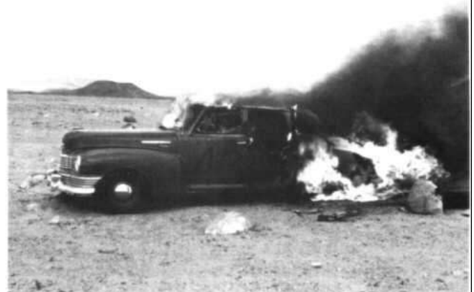
Fig. 7.2. Thermal radiation from a nuclear explosion entered the car above through its closed windows and ignited the upholstery. The windows were blown out by the blast a few seconds later. However, the explosion was at such a distance that the blast wave was not severe enough to dent the car body.
