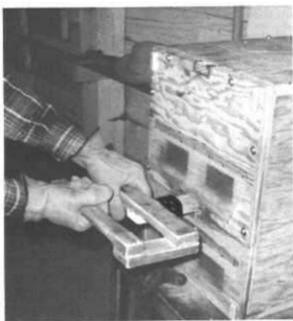
Fig. 16. (above) The Pump Handle of the Durability-Test Pump, showing how one man best holds it when two men are pumping.
