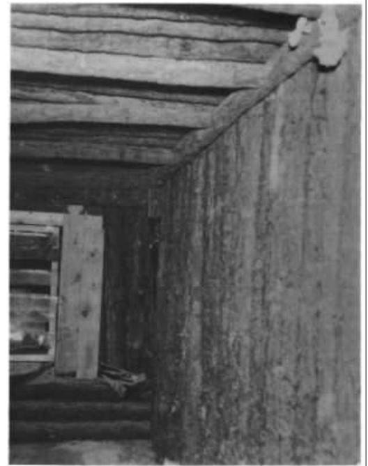
Fig. D.2. Undamaged interior of a Small-Pole Shelter after blast testing at the 53-psi overpressure range. Large buildings would have been completely demolished.
