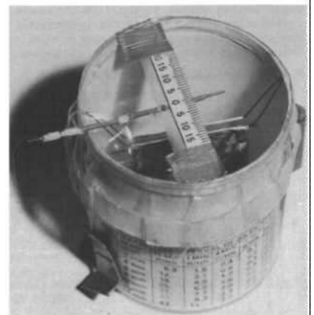
Fig. 10.1. A homemade KFM, an accurate dose rate meter for measuring dose rates from 30 mR/hr (0.03 R/hr) up to 43 R/hr.
