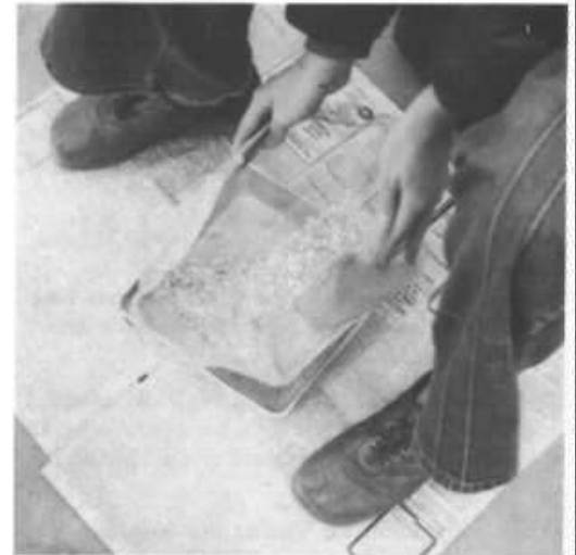
(Illustration)Fig. 9.1. Sieving ground barley through a window screen sieve.
