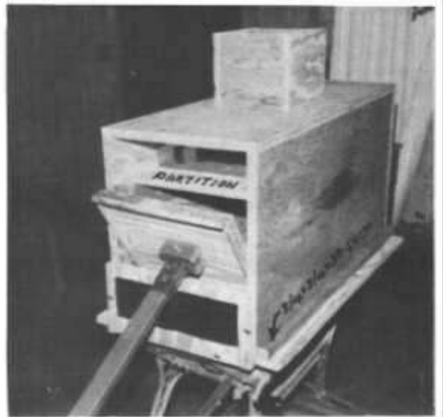
Fig. 6. Pump Built by Dale Huber, of Lake City, Florida in his home workshop, while guided only by the second draft of these repeatedly improved instructions. The removable part of the front end has been taken off, to insert the piston into the 12 x 12-in. "cylinder" under the PARTITION. The plastic flaps of this pump's flap valves are black: transparent plastic film is preferred.
